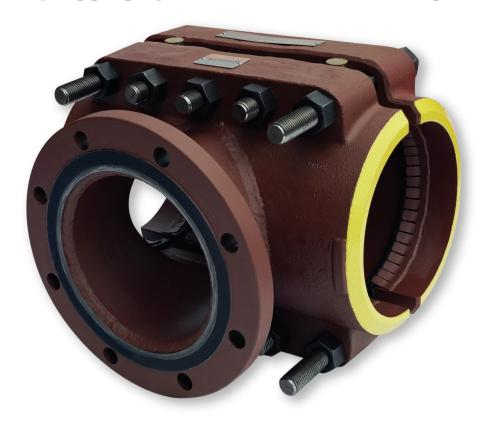
PLIDCO® Hot Tapping+Saddles are designed to ASME code section VIII and API 6H to make *branch connections* on existing pipelines OR for *plugging* operations without welding. They are easily installed by simply tightening the side bolts. Patented steel GirderRings hold seals in place to protect from damage and displacement during installation. When conditions are favorable PLIDCO® Hot Tapping+Saddles can be permanently welded to the pipeline.
